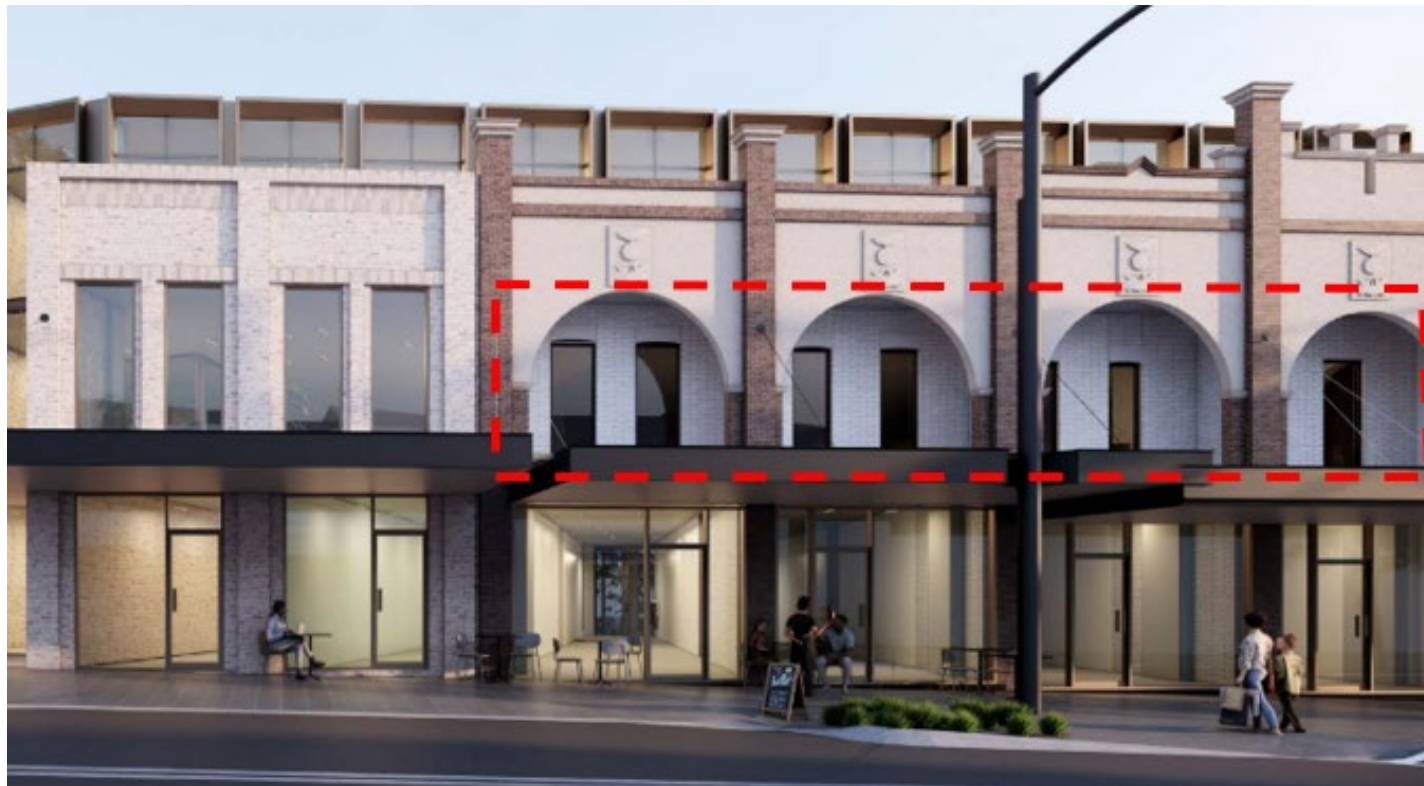
Perspective showing the retention of the existing balcony windows and walls of No.604-608 and reinstatement of the balcony and original windows of No.610
